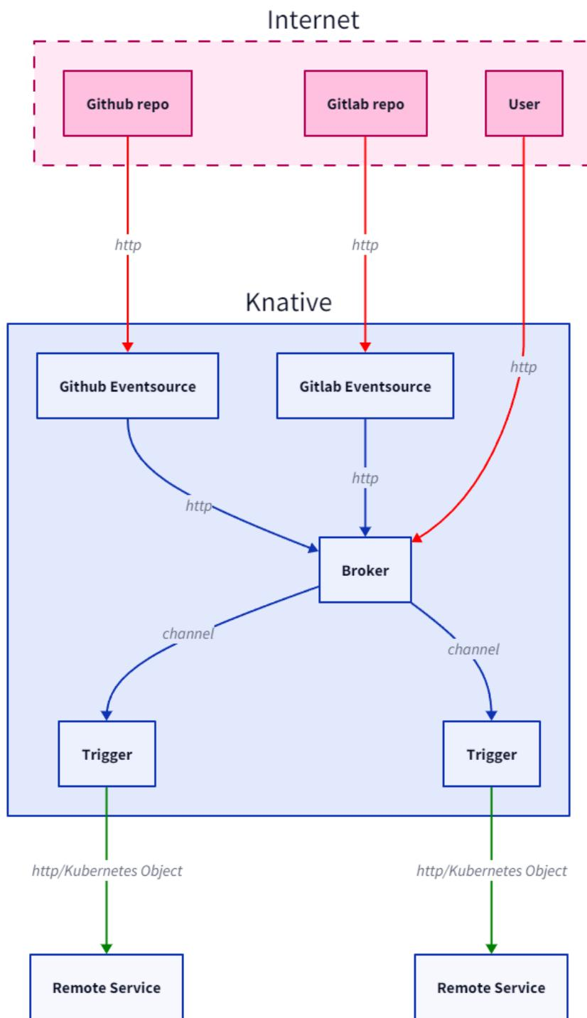
Figure 1.0.0: Trust and data flow of the Knative Event Mesh
