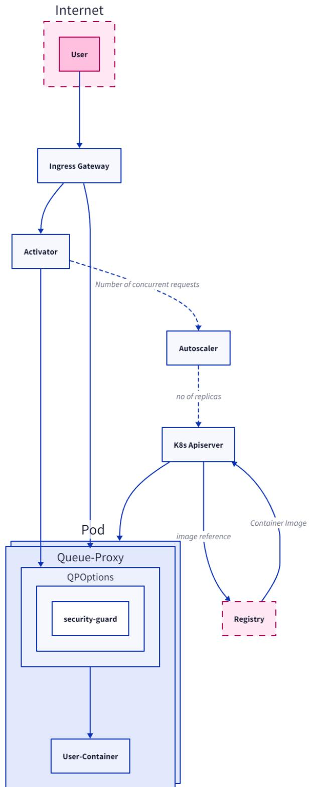
Figure 1.0.1: Trust and data flow of the Knative Serving
